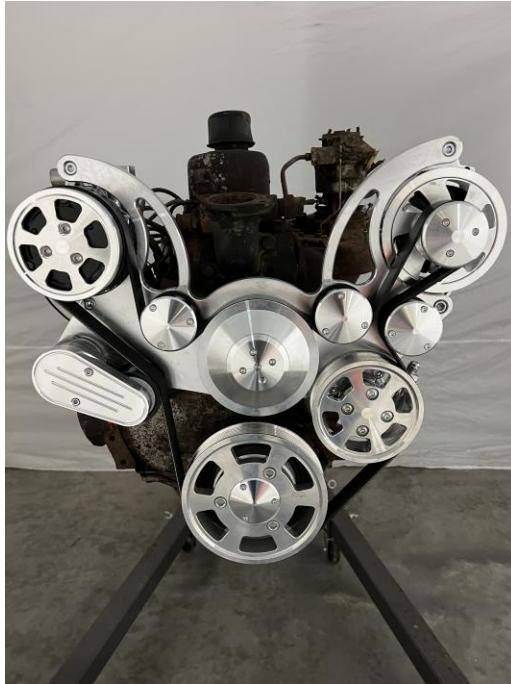
Step 13: Route the belt based on your configuration above. Recommended belts for proper tension are as follows:
