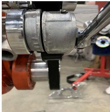
Step 15: If you are going to be running a mechanical fan, you will need to install FAN-SPACER-WR onto your water pump shaft.
