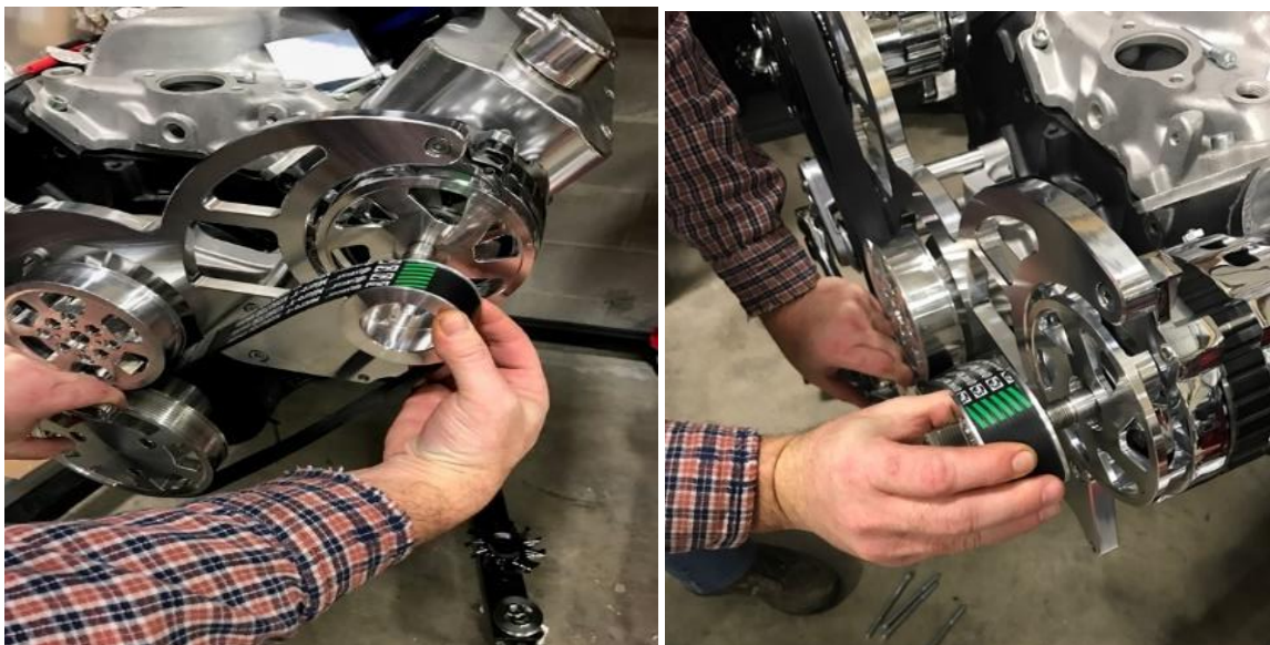
Belt Install with alternator pulley
