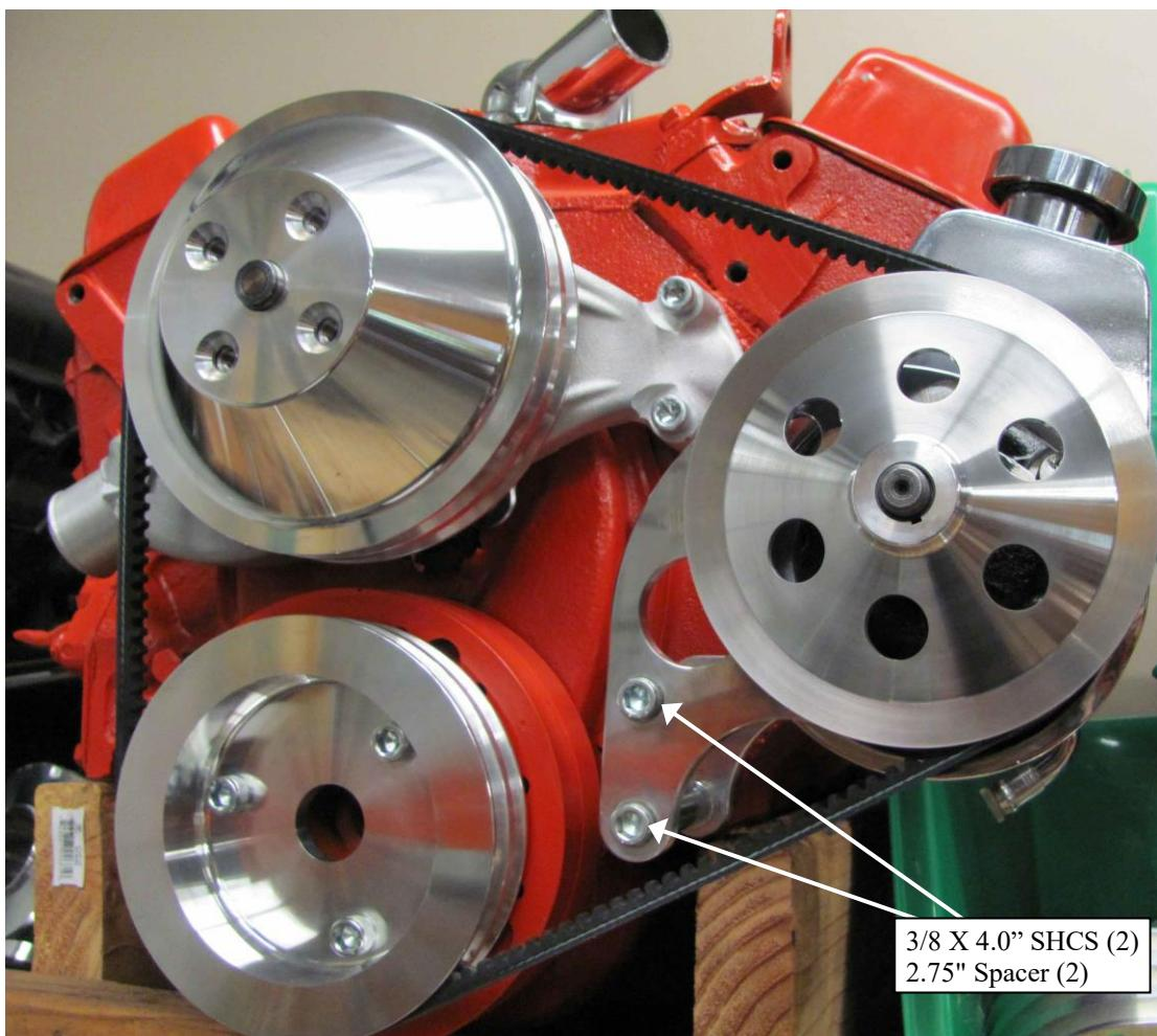
Step 1: Remove old power steering bracket.
