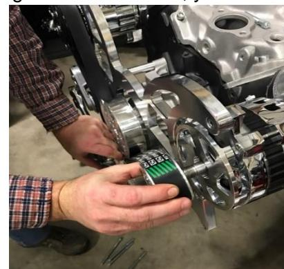
need to install FAN-SPACER-WR onto your water pump shaft.
