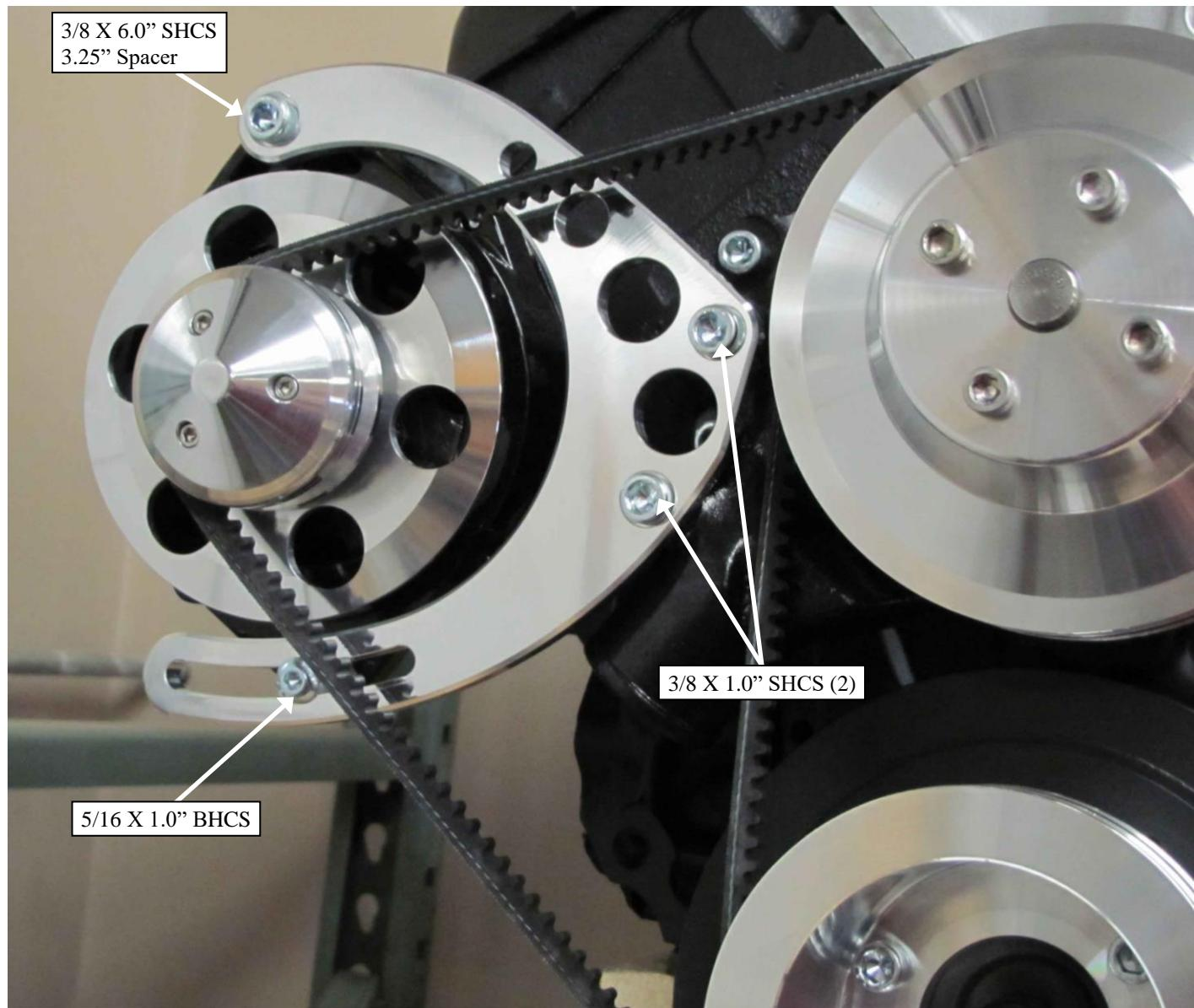
Step 1: Remove old alternator bracket.
