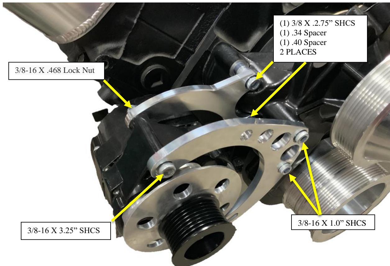
Step 1: Remove old alternator bracket.
