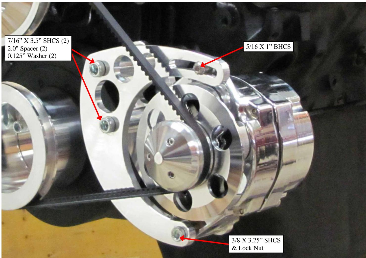
Step 1: Remove old alternator bracket.
