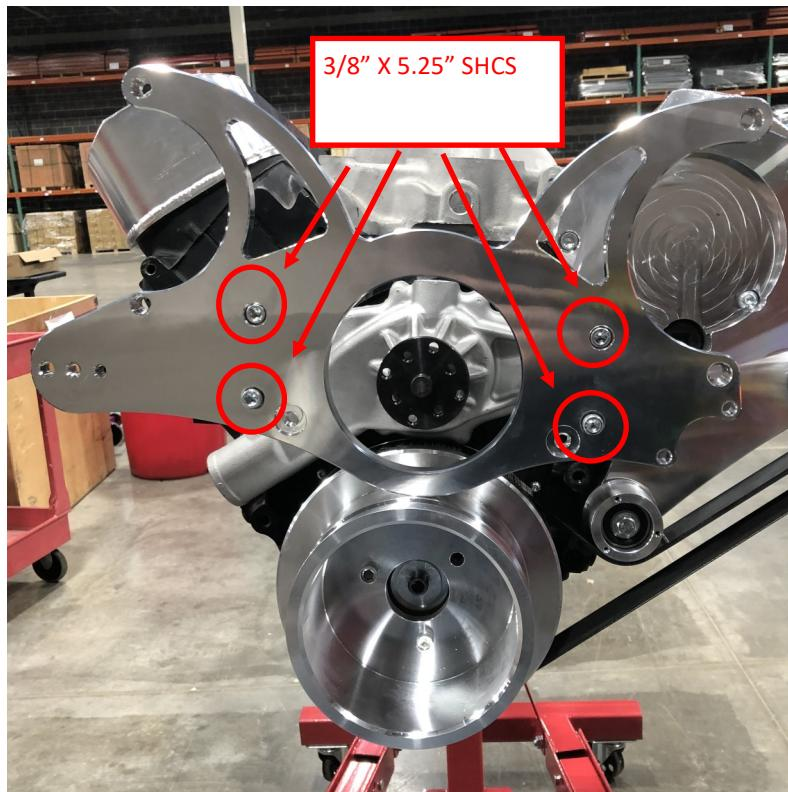
9. Install the alternator (**CS130-1WIRE-140A**). You will want to remove the stock steel fan and alternator pulley before continuing.
