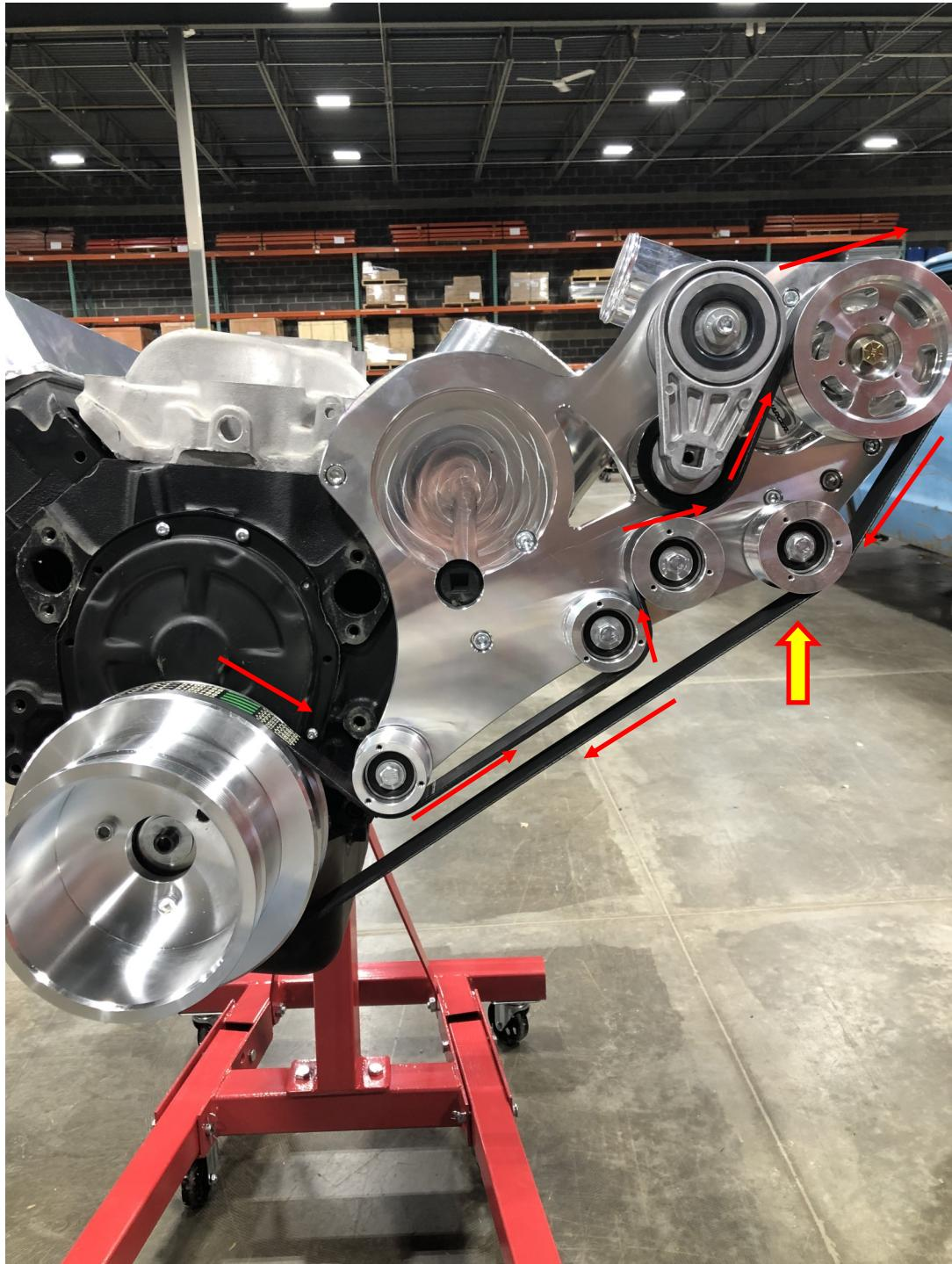
7. Route the 10 rib belt supplied with your kit ([K100789](#)) as seen in the image to the route. The idler with the thick yellow arrow will be the final piece you route. This step may be easier with someone to help pull the tensioner back, but can be done alone.
