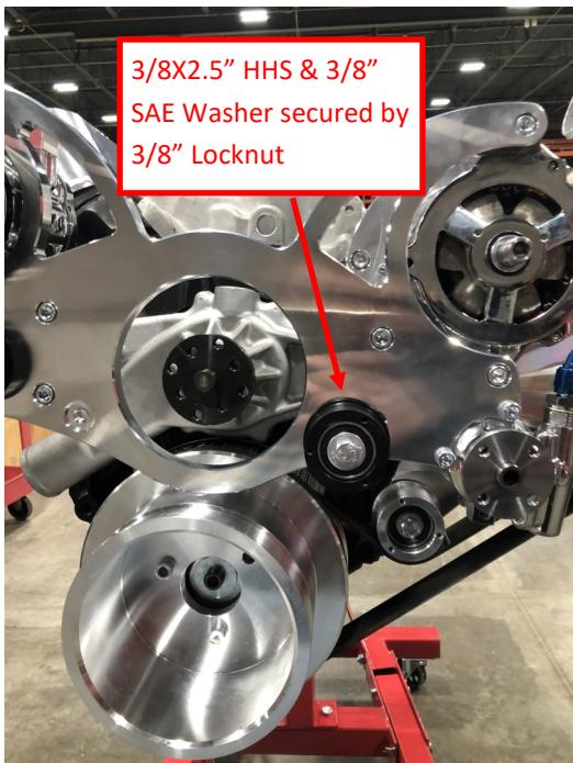
12. Install the tensioner ([TENSIONER-KIT](#)). You will use the 3/8 X 3" BHCS and a 3/8" Locknut. Again, it is recommended to keep the cap on the side until the belt is routed.
