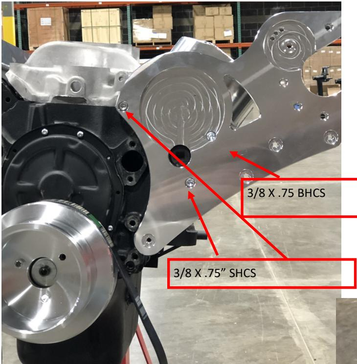
1. Begin by installing the Procharger plate (454-WR-PC). You will use (2) 3/8 X 1.25" SHCS and (1) 3/8 X .75" BHCS. These can be tightened to spec once all 3 bolts are started.
