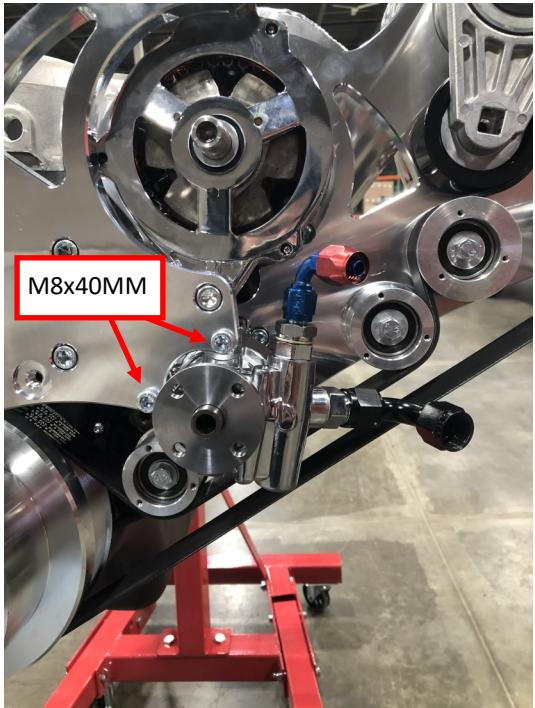
10. Install your power steering pump ([GM-TYPE2-PUMP](#)) or ([KRC-PUMP](#) and [HYDRO-BRACKET-KIT-WR](#) for hydroboost applications). The power steering pump is secured with both M8 X 40MM bolts.
