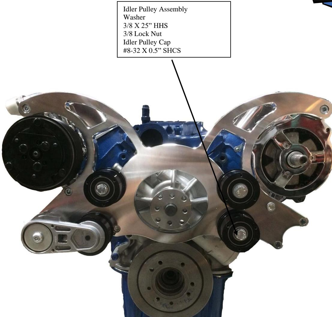
Step 1: Remove old brackets pulleys and water pump (if applicable)
