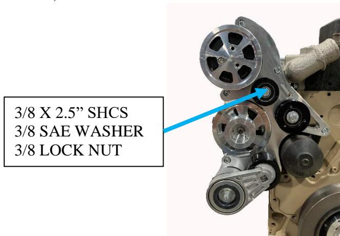
**Step 9:** Install upper main bracket bolt for added support. There are two different ways in doing this. If you have a 12-valve head please follow Step 9A. If you have 24 valve/common rail head, follow step 9B.
