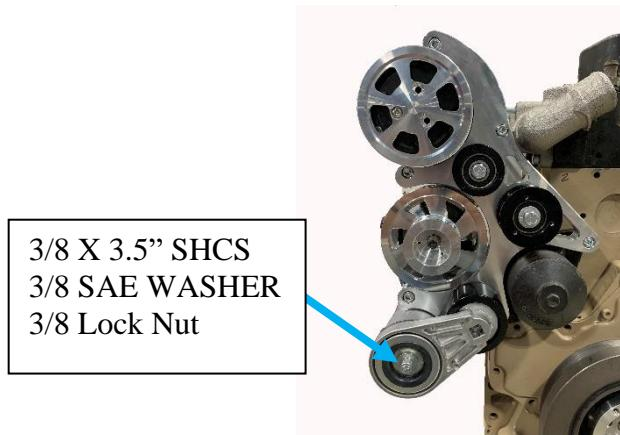
**Step 8:** Install smooth idler pulley (SERP-IDLER-WR) onto main bracket with One 3/8 X 2.5" HHS, one 3/8 SAE washer & One 3/8 Lock Nut.(pulley, pulley cap and cap hardware will be in the separate SERP-IDLER-WR box.)
