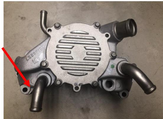
Step 2: You must rotate the shown hose connection to allow for bracket clearance.
