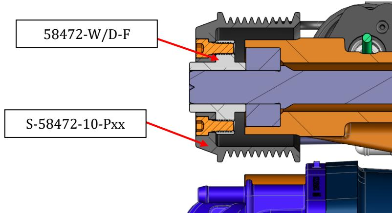
7. Install the hub adapter, 10 rib crank pulley, and 8 rib crank pulley. Bolts will be in the pulley and hub boxes
