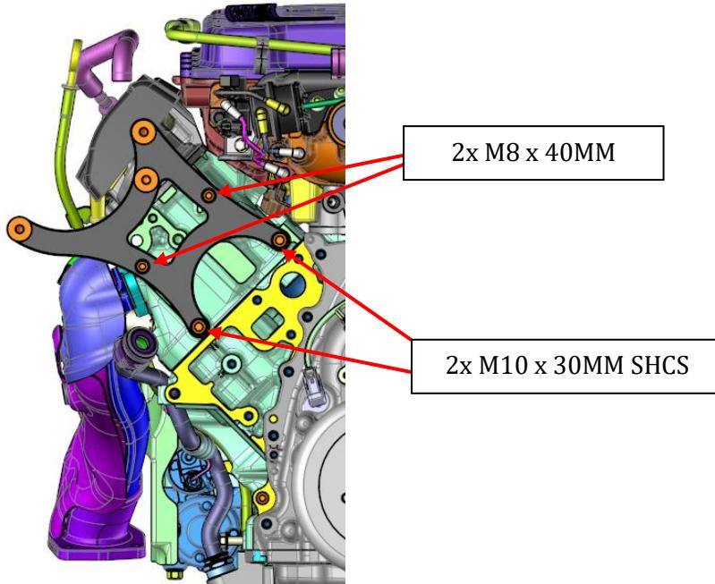
c. Mounting hardware can be found in box LT4AC-SC2-RP+
