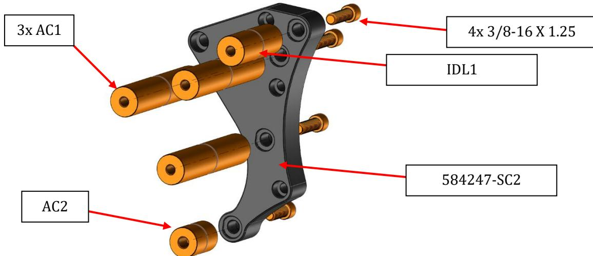
2. Assemble the pre-assembled rear support brackets to the engine
