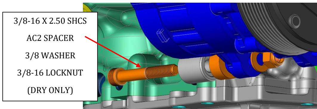
13. Install the alternator. Mounting bolts can be found in box LT4ALT-SC2-RP. Tighten all bolts including the 2 in the bracket from Step 10
