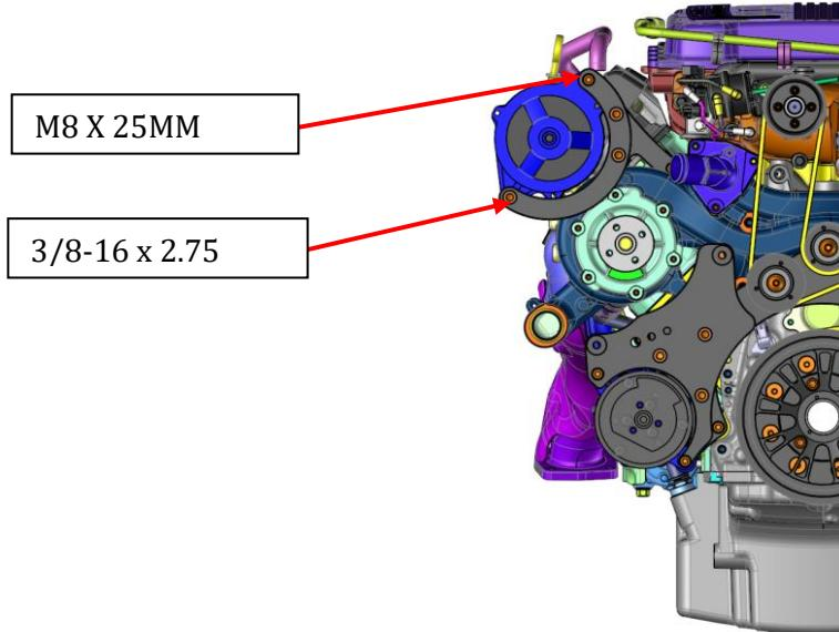
14. Install the PS Pump. Mounting bolts can be found in box LT4PS-SC2. Tighten all bolts. If you have a kit without a PS Pump, install the PS-Delete kit.
