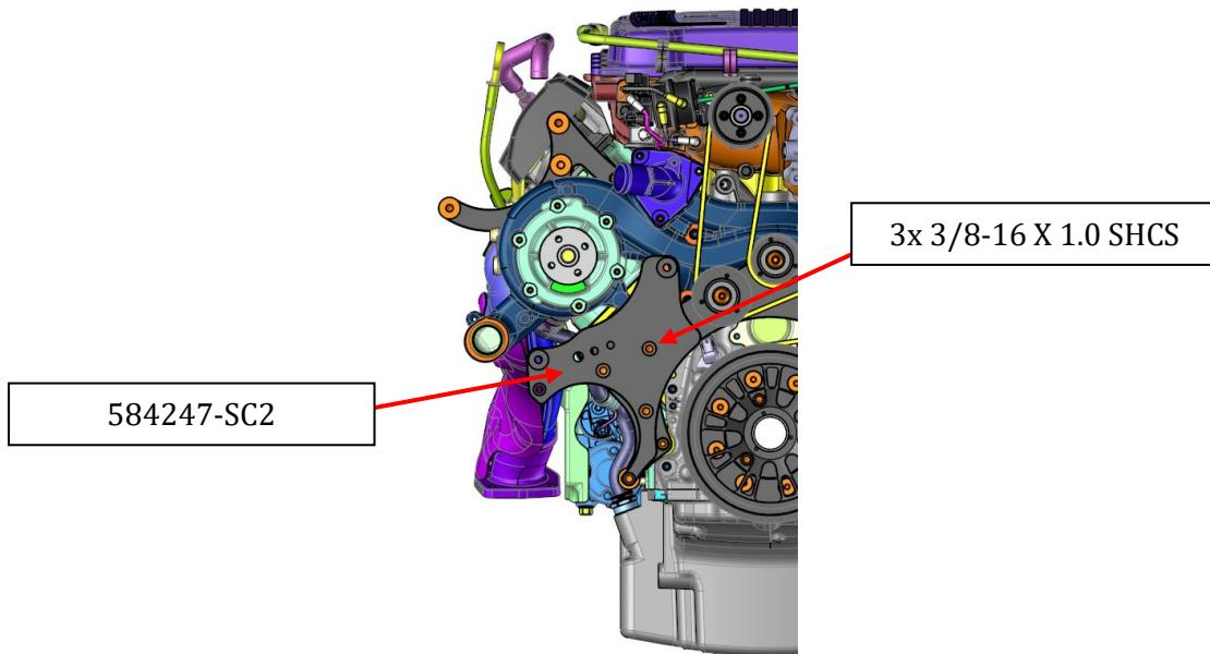
10. Mount the Front ALT Bracket to the spacers. Bracket and mounting bolts can be found in box LT4ALT-SC2-RP. Leave the bolts slightly loose
