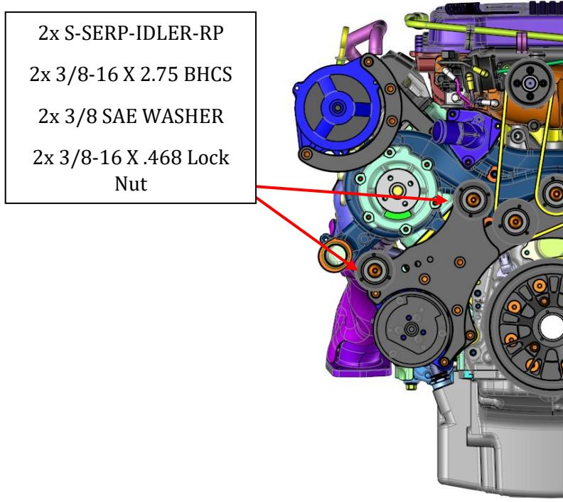
16. Install the Alt Fan and Pulley (installation nut is on the alt shaft). Install the water pump pulley with included bolts in the pulley box. Install PS pulley with the included bolts in the pulley box.
