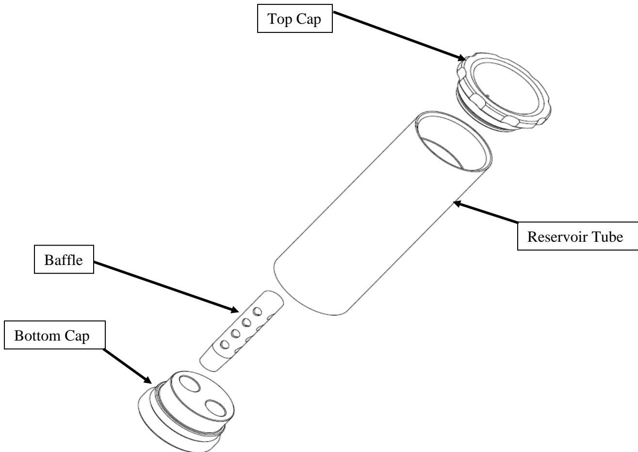
Step 2: Install O-Rings on top and bottom caps. Carefully tighten by hand without marking the surface.
